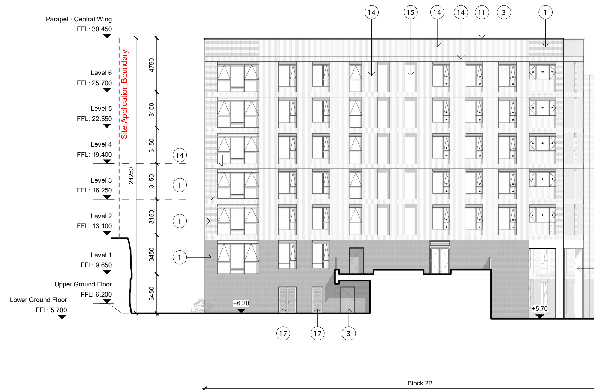
3 Block 2B - Central Wing - West Elevation 1 : 200
