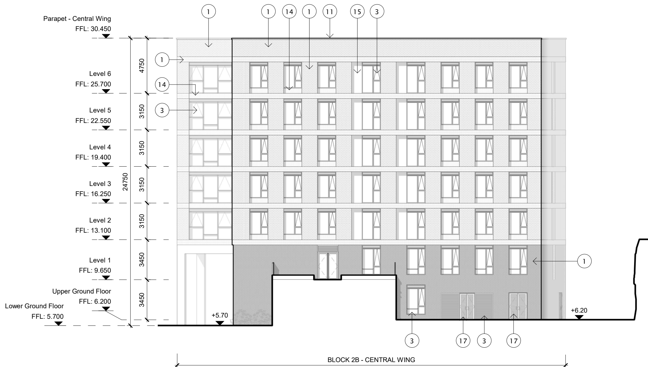
1 Block 2B - Central Wing - East Elevation 1 : 200
